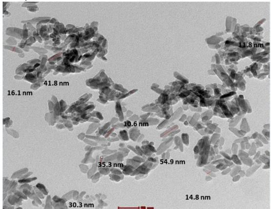
Fig.2. TEM image of HA-NPS powders synthesized.
