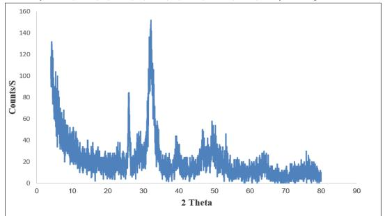
Fig.1. XRD patterns of hydroxyapatite (HA) powders synthesized.
