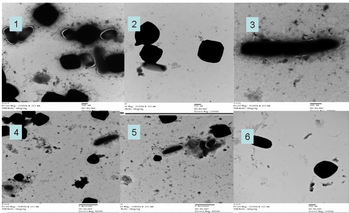
Fig. 5: *Spli*NPV virus in combination with nano aluminum oxide (2, 4, 5) or nano zinc oxide under scanning electron microscope (1, 3 and 6).
